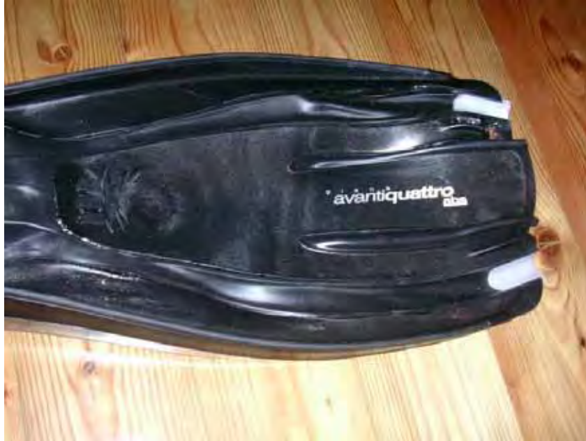
This fin was subject to high temperature
